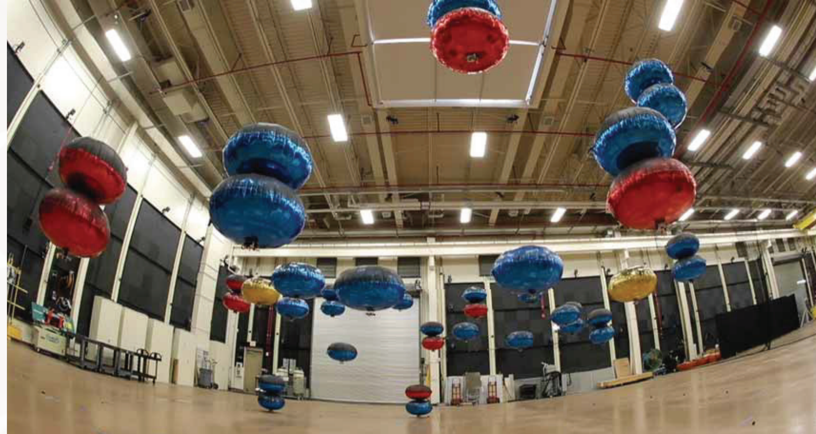
Researchers at the U.S. Naval Research Laboratory have developed a fleet of autonomous platforms to test the swarming behavior of autonomous systems. They successfully demonstrated the operation of 30 blimps in December 2018. This year they aim to fly more than 100 controlled balloons (also known as miniature autonomous blimps).
